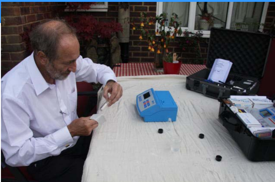
Figure 5 - Cleaning the cuvettes. Maintaining the cuvettes in pristine condition is vital for accurate water testing.
